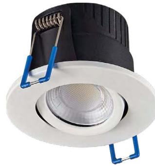
IP20 / IP65 façade IK08 DIM TRIAC 60° 25° Ø68 - 74 mm TOUT ISOLANT IRC>80 Classe II 50 000 h (L70)
